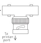
3 Attach another section of thin-wire Ethernet cable or a 50 ohm terminator to the other end of the BNC "T" connector.
